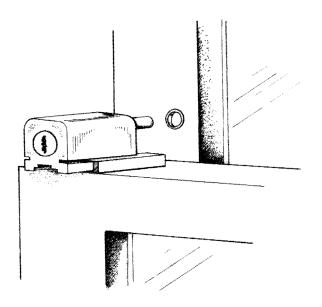
Auxiliary latches may also be installed. The most effective protection for double-hung windows is a key-locking security sash lock. If possible, mount the lock with two-inch wood screws.
