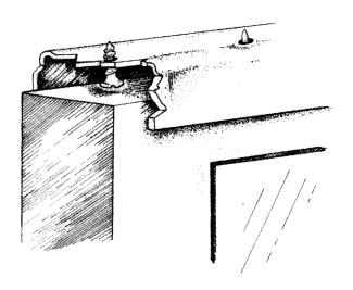
A supplemental lock should be installed at the top or bottom, made out of steel and inserted in the sliding door at a slightly downward angle.
